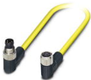
Sensor/Actuator cable, 4-position, yellow, Plug angled M8, on Socket angled M8, Cable length: 1.5 m
