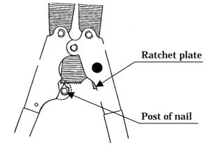
The post of the nail finally bumps to the ratchet plate.
