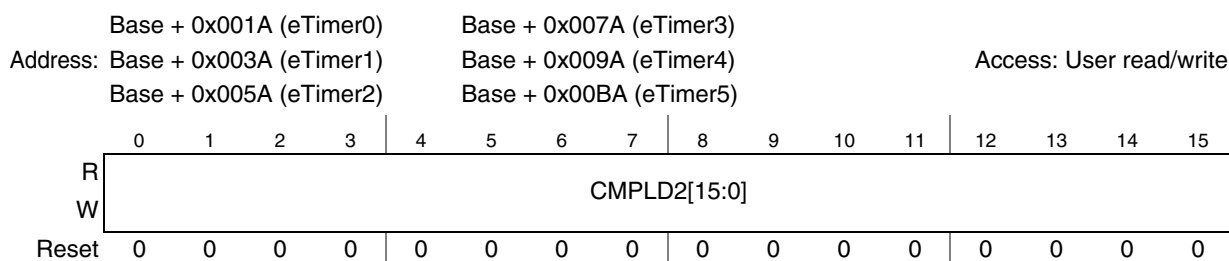
Figure 405. Comparator Load 2 (CMPLD2)
