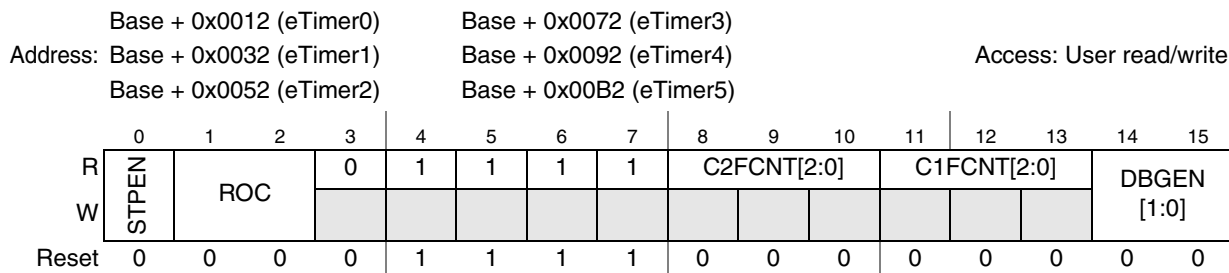
Figure 401. Control register 3 (CTRL3)
