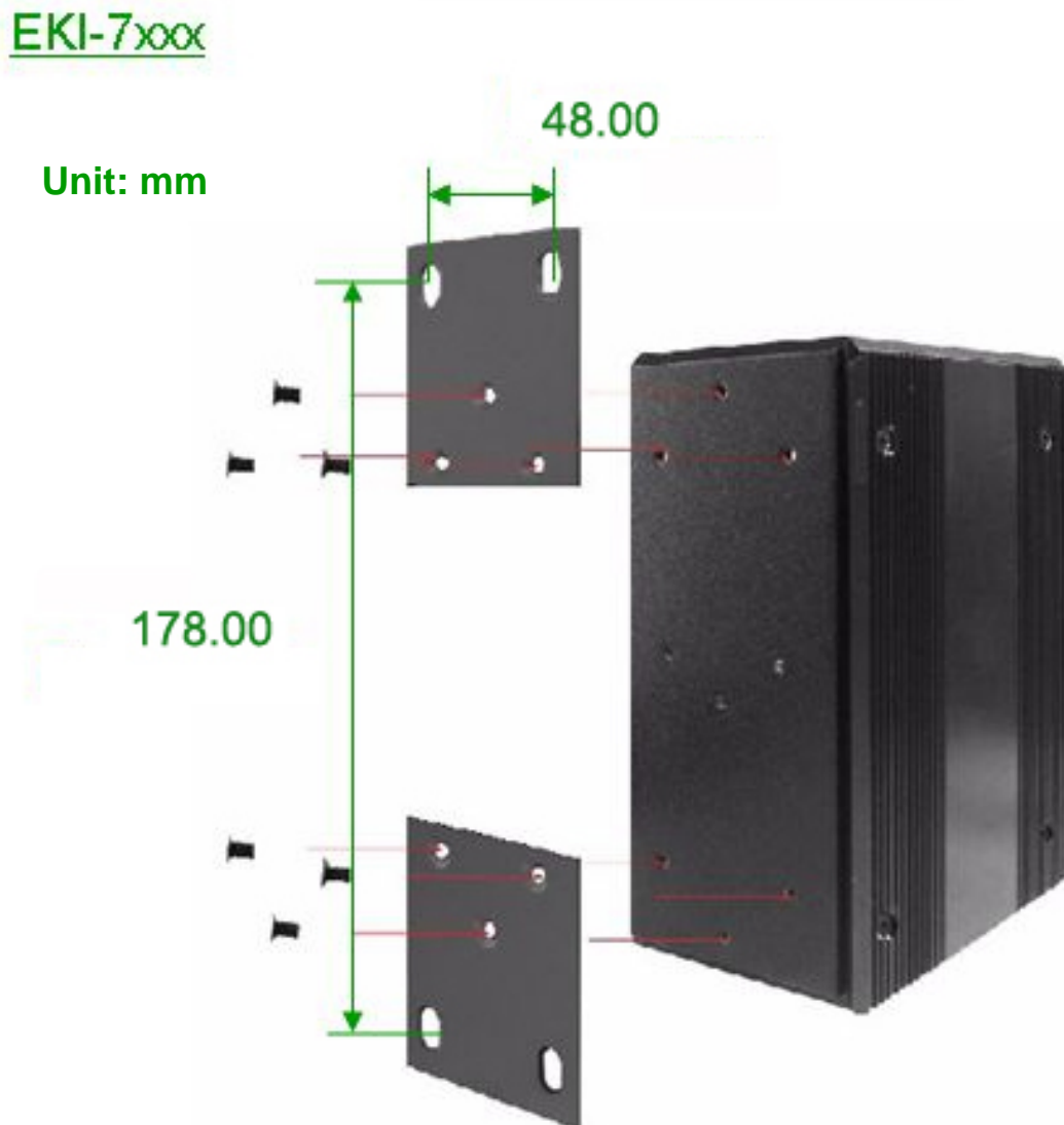
Figure 2.5: Combine the Metal Mounting Kit
