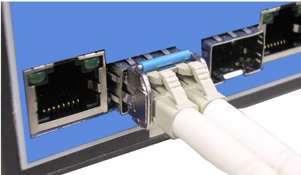
Figure 2.10: LC connector to the transceiver
