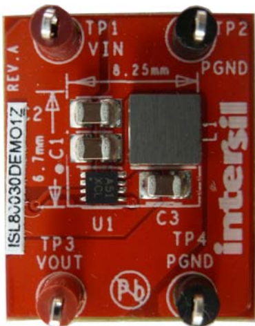
FIGURE 2. ISL80030DEMO1Z TOP SIDE
