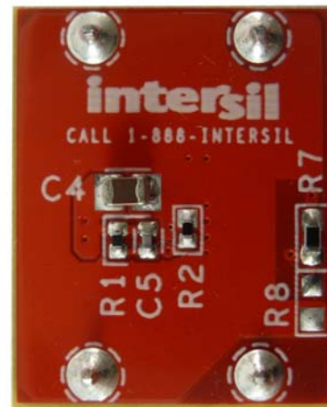
FIGURE 3. ISL80030DEMO1Z BOTTOM SIDE
