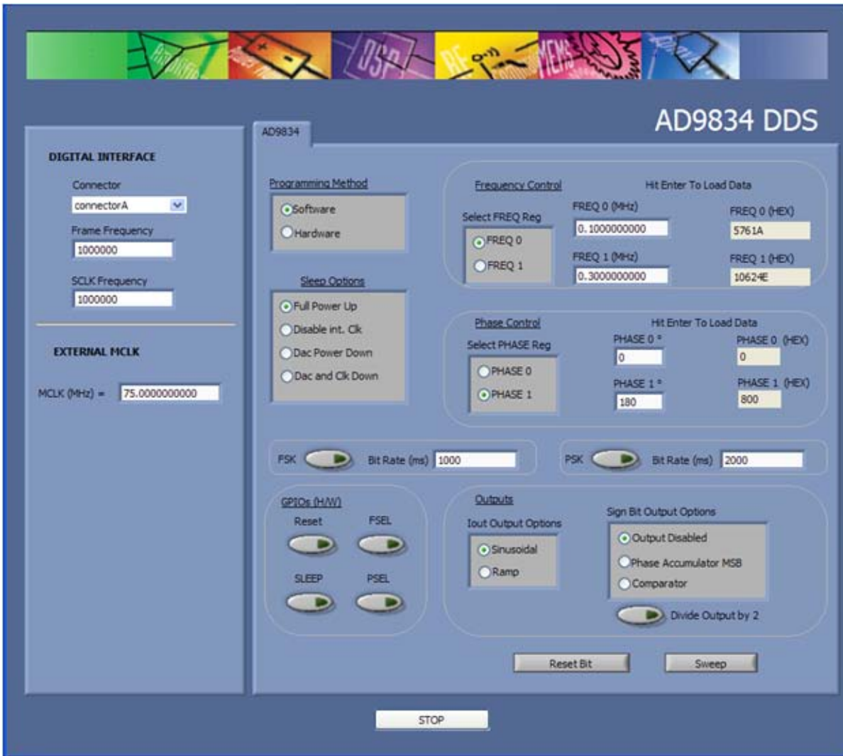
Figure 4. AD9834 Evaluation Board Software
