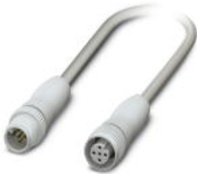
Sensor/Actuator cable, 5-position, PP-EPDM halogen-free, Gray RAL 7035, Plug straight M12, A-coded, on Socket straight M12, A-coded, Cable length: 0.3 m, Hygienic design, with plastic knurl
