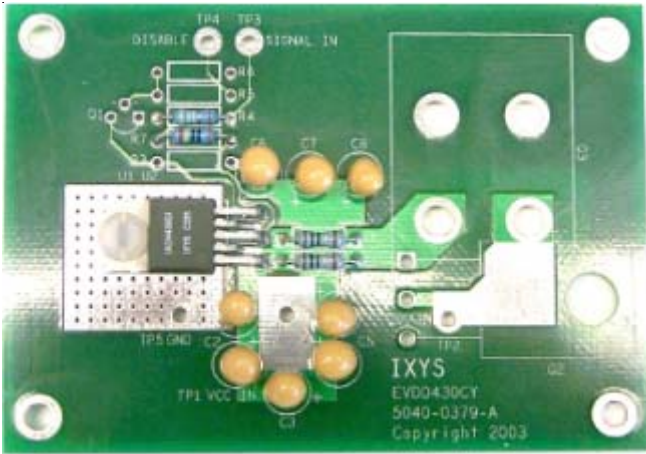
Figure 1 EVDD430CY Evaluation board with 5 lead TO-220 driver installed.
