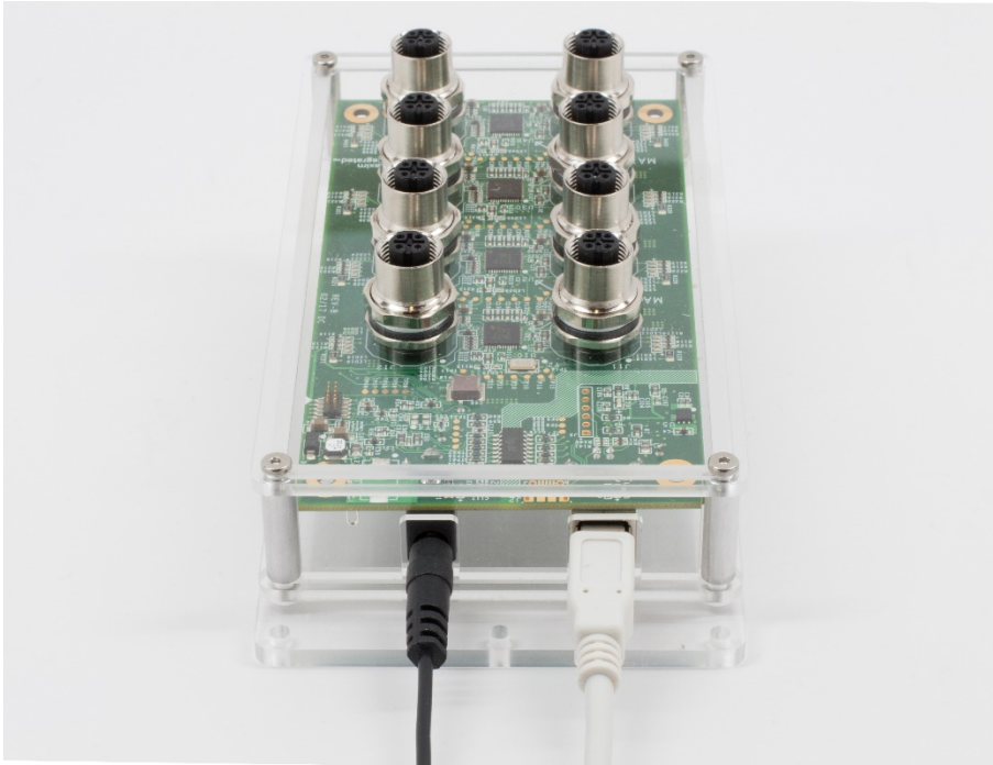
Figure 4. Connect the Power and USB cables to MAXREFDES145# and then connect it to the PC.
