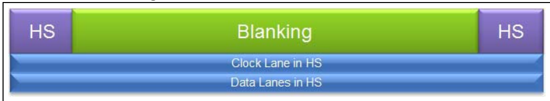
Figure 199. Clock lane and data lanes in HS
