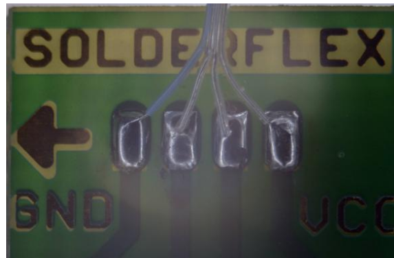
Figure 6: NanEye's 4-Pin Connector Soldered Wires
