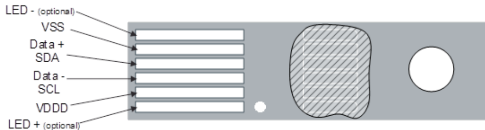
Figure 3: NanEye's 6-Pin Flex PCB Connector Pinout
