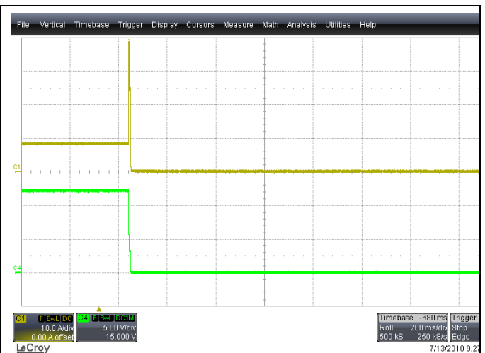
Figure 33 - Latching short circuit protection, 60VDC Upper trace: Output current, 10A/div, 500ms/div Lower trace: Output Voltage, 5V/div, 500ms/div
