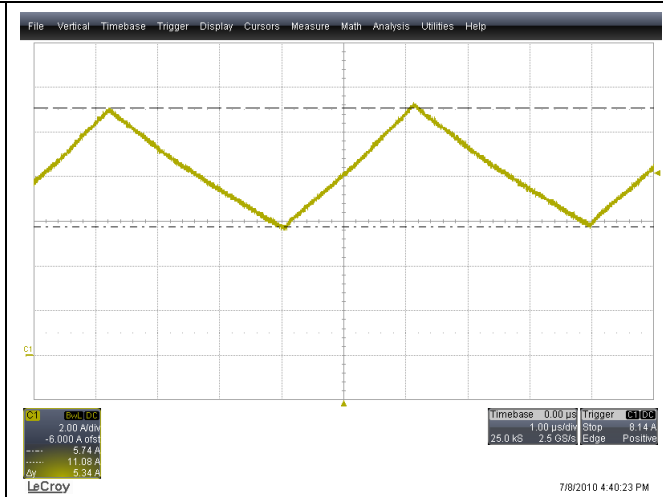
Figure 75 - Output inductor current, 60VDC, 8A load, 2A/div, 1µs/div
