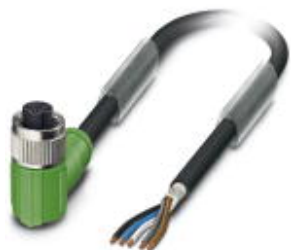
Sensor/actuator cable, 5-position, Variable cable type, shielded, free cable end, on Socket angled M12, A-coded, cable length: Free input (0.2 ... 40.0 m)
