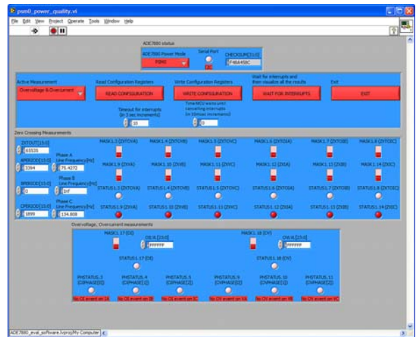
Figure 27. Overvoltage and Overcurrent Measurements Panel
