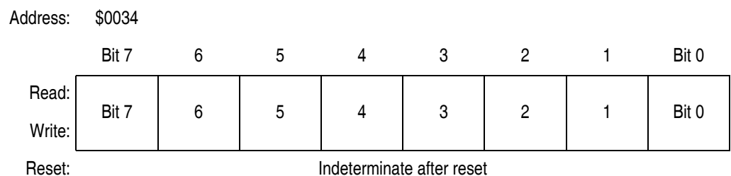
Figure 12-19. TIMB Channel 2 Register Low (TBCH2L)
