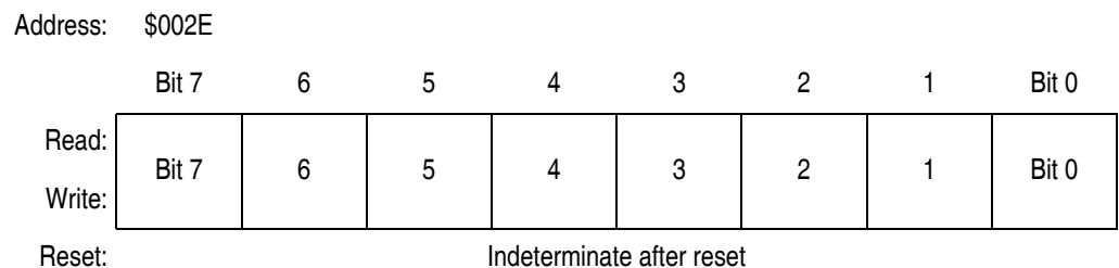
Figure 11-19. TIMA Channel 2 Register Low (TACH2L)
