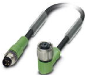
Sensor/actuator cable, 4-position, Variable cable type, Plug straight M8, on Socket angled M12 SPEEDCON, A-coded, cable length: Free input (0.2 ... 40.0 m)
