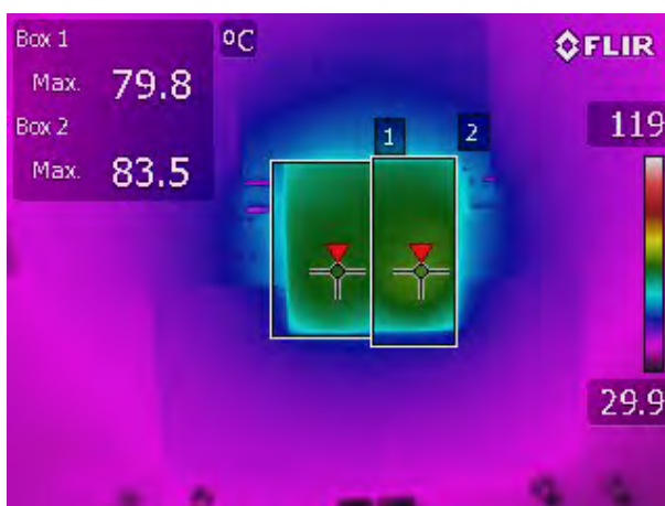
Figure 11. Thermal at V_{IN} = 12V , V_{OUT0} = 1.0V , I_{OUT0} = 18A , V_{OUT1} = 1.8V , I_{OUT1} = 18A , T_A = 25^\circ C , 200LFM Airflow
